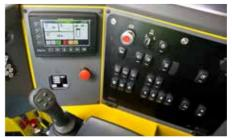
Scooptram ST14 S has a smart control system featuring traction control. speed limiter, over speed protection and automatic delivers exceptional reliability, cost of
