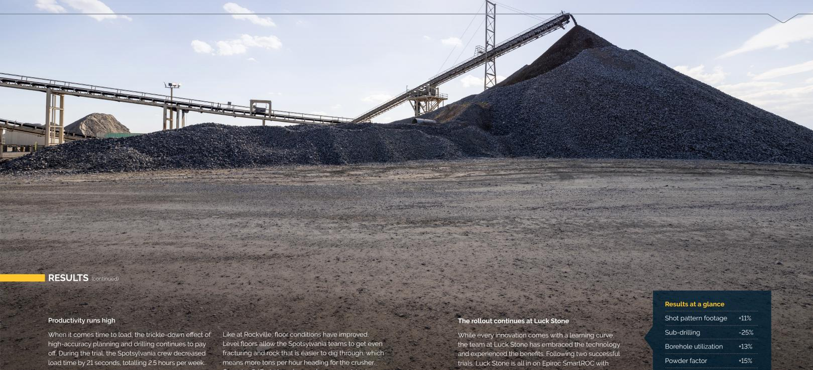
At the crusher, Spotsylvania saw a +14% increase—that's almost 100 tons an hour—in throughput as measured in tons per hour run (TPH-R). Black belt time decreased by 5% and the team estimates a ~25% decrease in the amount of oversize rock that requires secondary breakage. Incredibly, a hydraulic rock-breaker that has worked full-time at the site for years has now been able to leave the site for brief periods since the material is now rightsized for the primary crusher.
